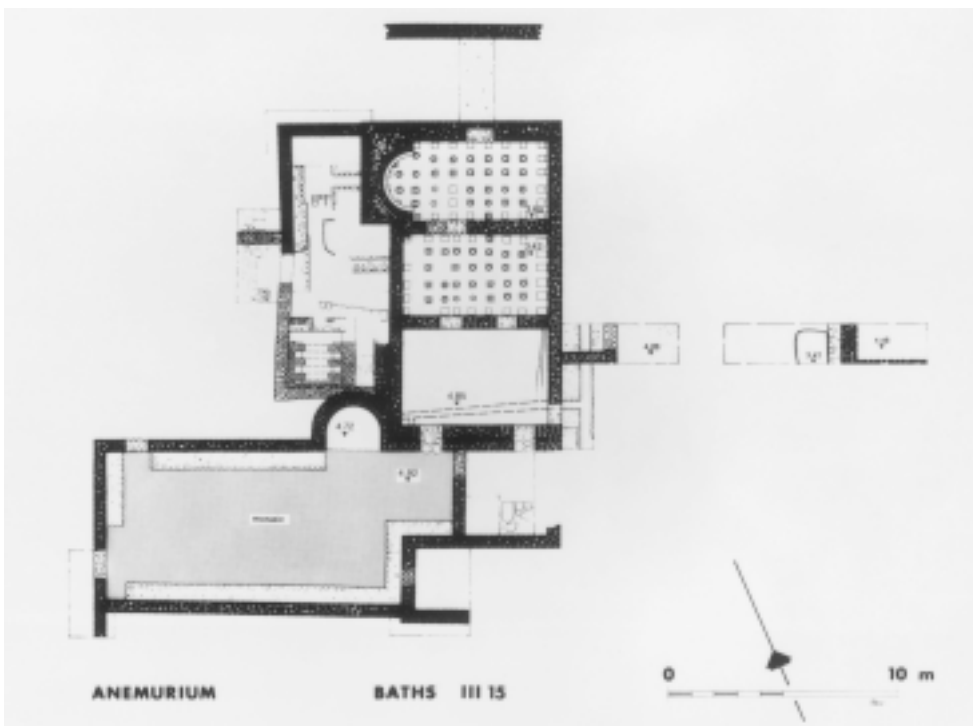
4. Anemourion, plan of small Byzantine baths adapted for commercial purposes in the city's latest phase (drawing by Tom Boyd)
